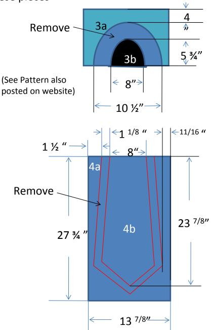
Use ½" Particle Board or Plywood for these 2 identical pieces (not to scale)
