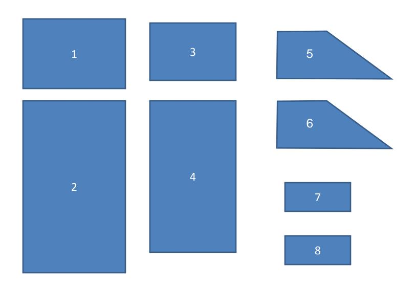
Use Exterior Grade Particle Board or plywood for all parts. Everything gets soaked as you spray water over/through the PVC when bending the frames. Suggest you also apply several coats of lacquer or other waterproofing finish.
